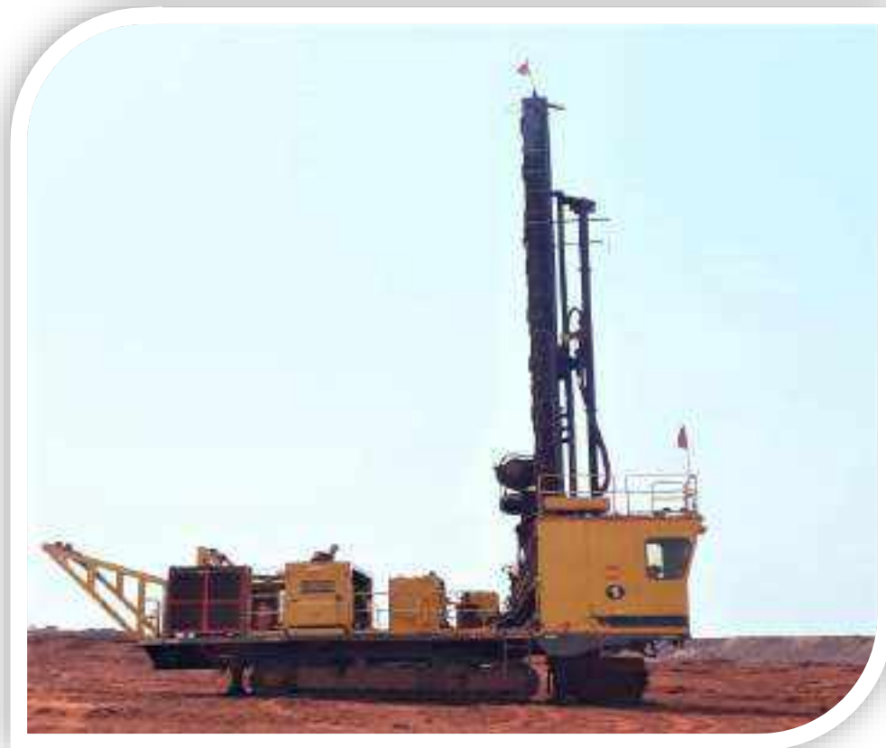
PHOTO 11: Showing drilling machine with dust Extractor
