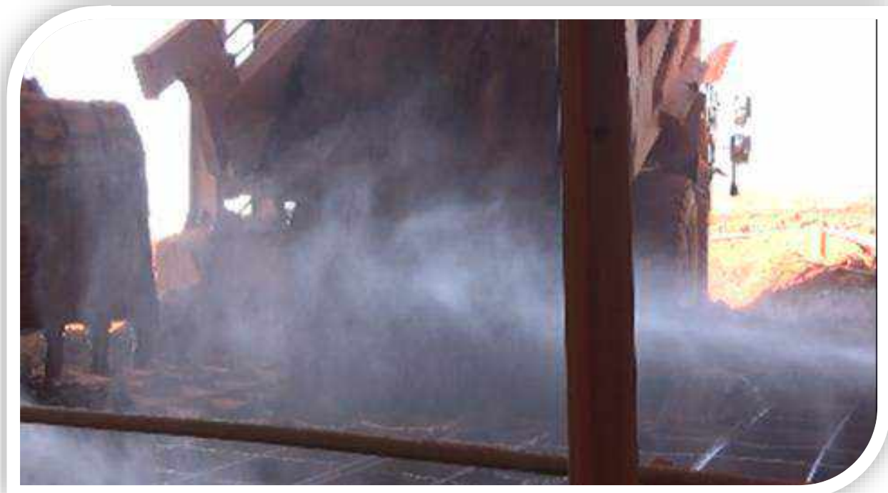
PHOTO 13: Showing Dry fog system in Fixed Crushing plant
