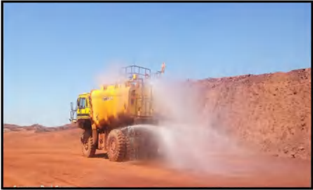
PHOTO 8: Showing 28KL Mobile sprinkler
