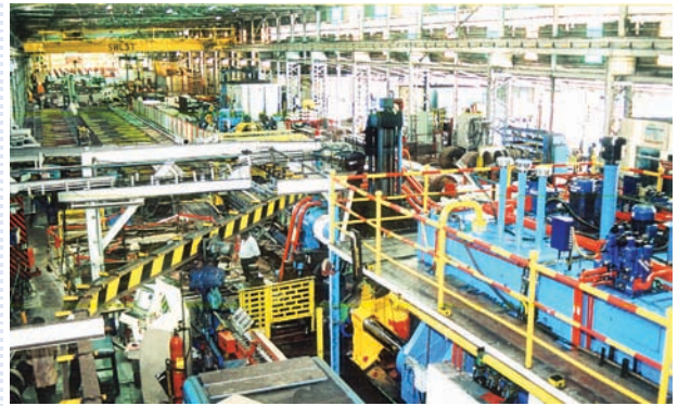
3300 T Farrel Watson Stillman Press with 9" & 12" containers, automatic controls and puller
