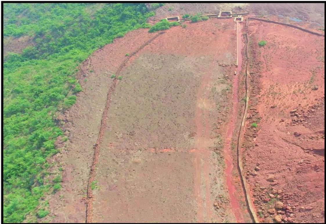
PHOTO 2: Showing Retaining wall & garland Drain along the Dump Slope
