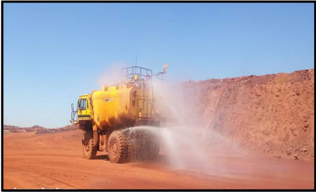
PHOTO 8: Showing 28KL Mobile sprinkler
