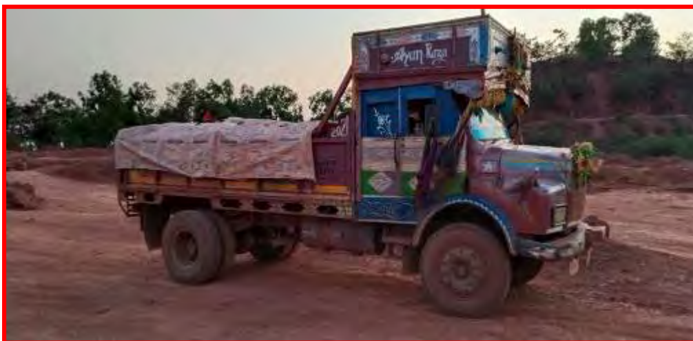
Tarpaulin covering during material loading-unloading
