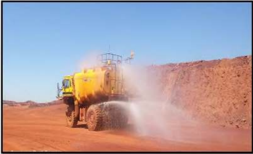
PHOTO 8: Showing 28KL Mobile sprinkler
