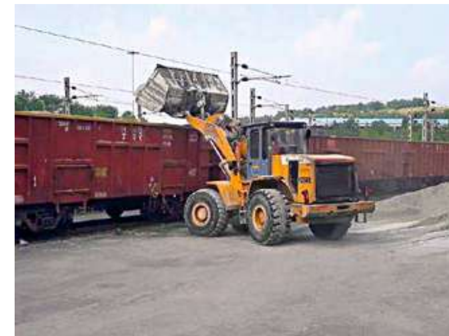
A fly ash rake is loaded at a Hindalco unit for transporting to a cement plant. Fly ash transfer by railway is easier on the environment
