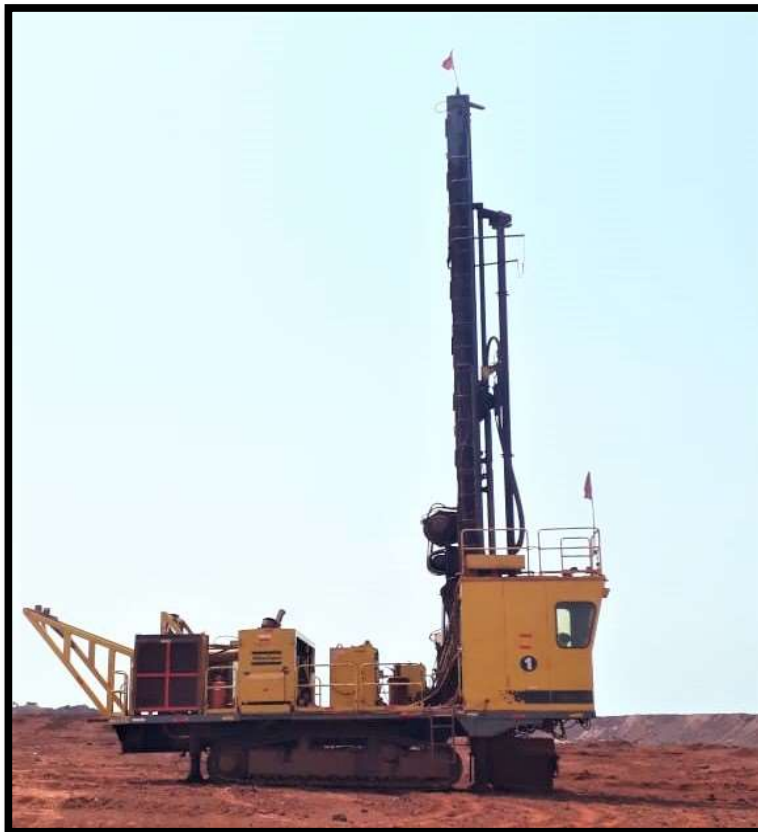
PHOTO 11: Showing drilling machine with dust Extractor
