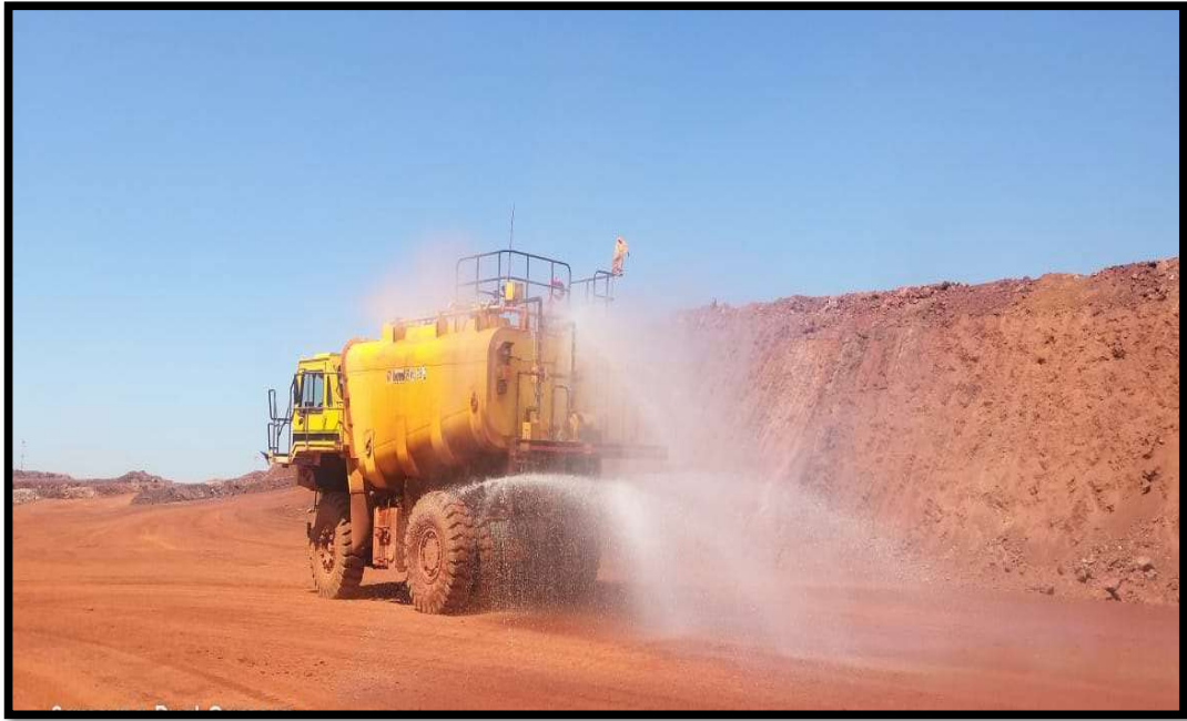
PHOTO 8: Showing 28KL Mobile sprinkler
