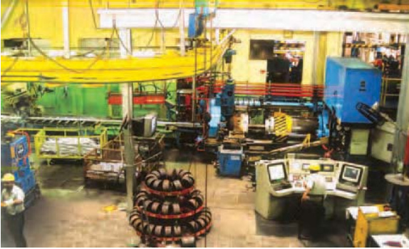
1250 T Lowey Hydraulic Press with 6" container, automatic controls and puller
