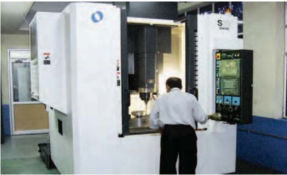
Ultramodern Makino Vertical Machining Centre in Die Shop
