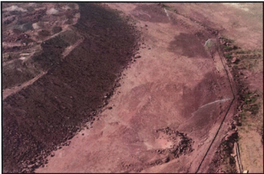
Photo -10 : Showing Fixed water sprinklers around stock pile area
