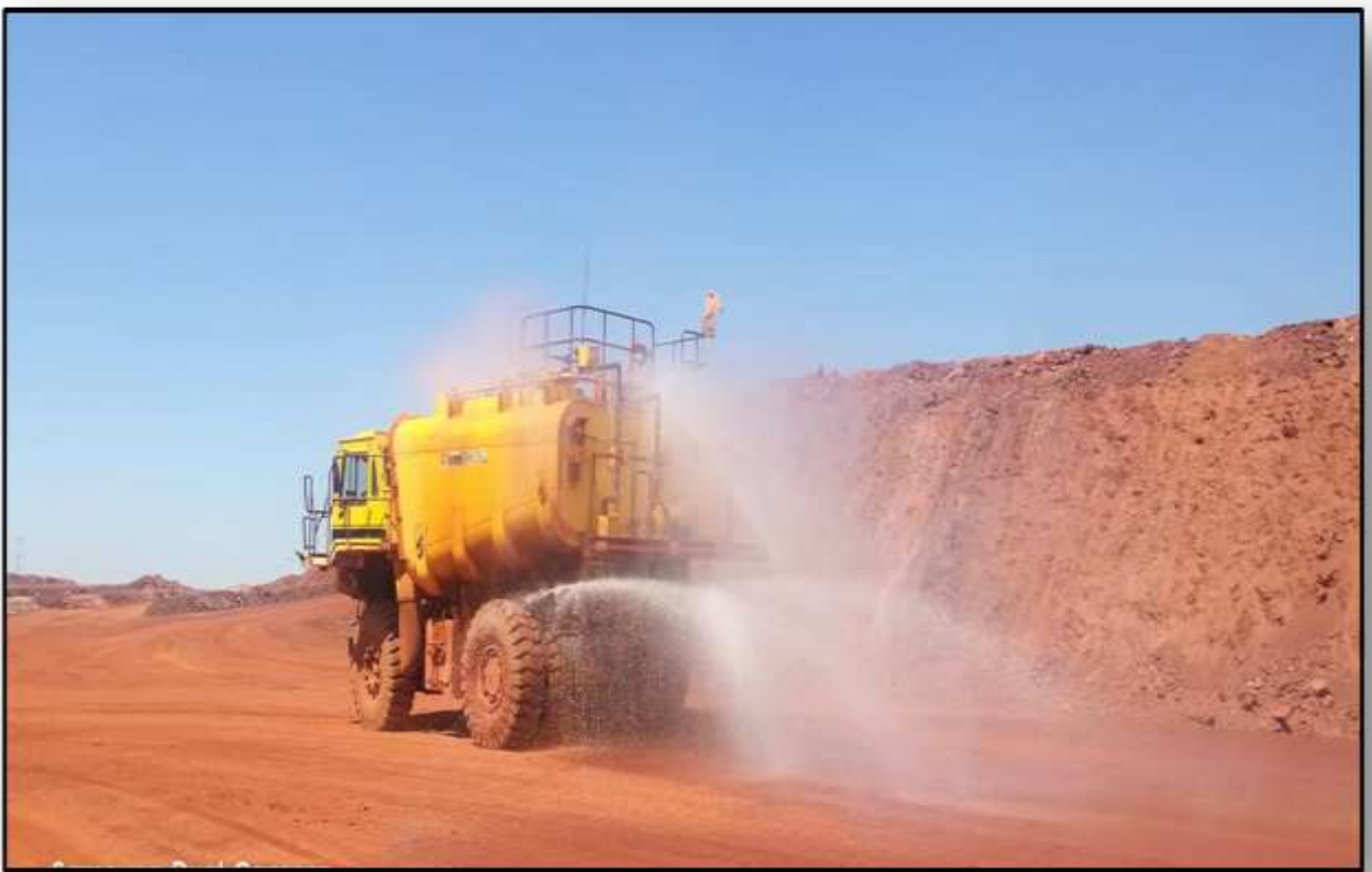
PHOTO 8: Showing 28KL Mobile sprinkler
