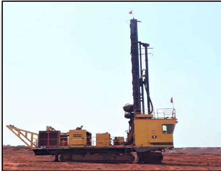
PHOTO 12: Showing drilling machine with dust Extractor.
