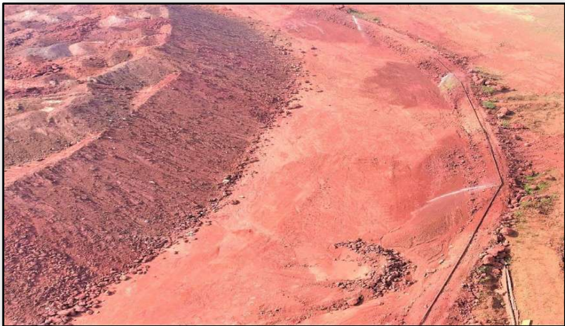
PHOTO 13: Showing Fixed sprinklers in stockpile area.
