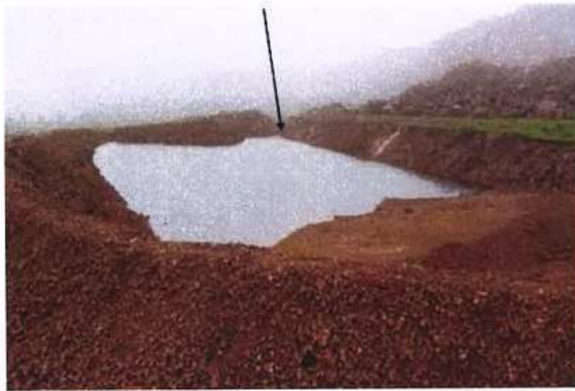
Figure 8: Settling pond near Rayagada dump.
