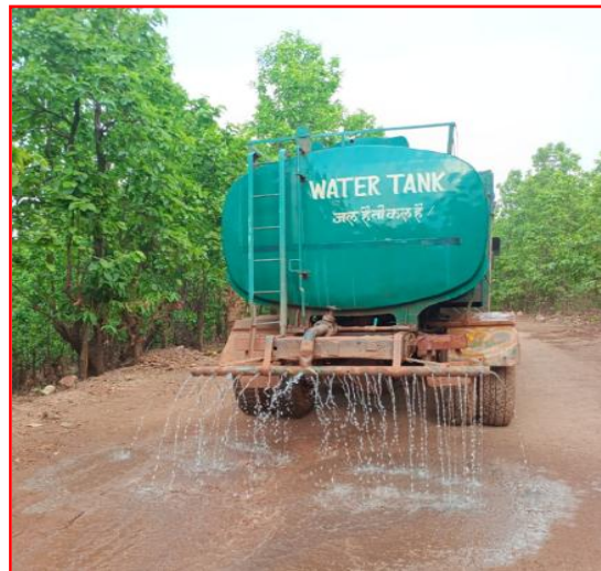
Mobile Water Tanker with Sprinkling Facility
