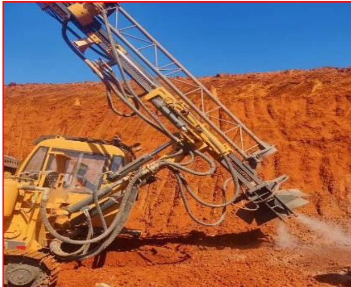
Wet drilling is in practice.
