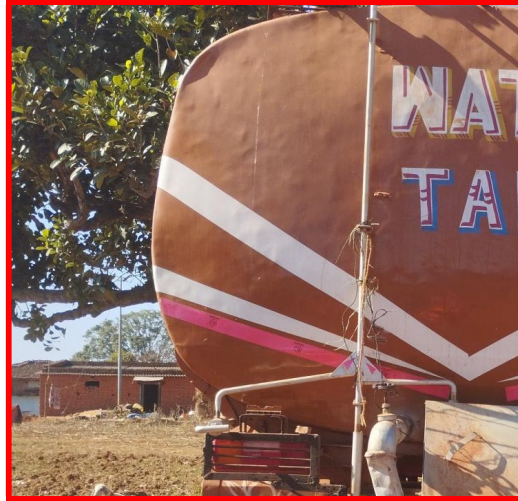
Dust Suppression through water tanker.
