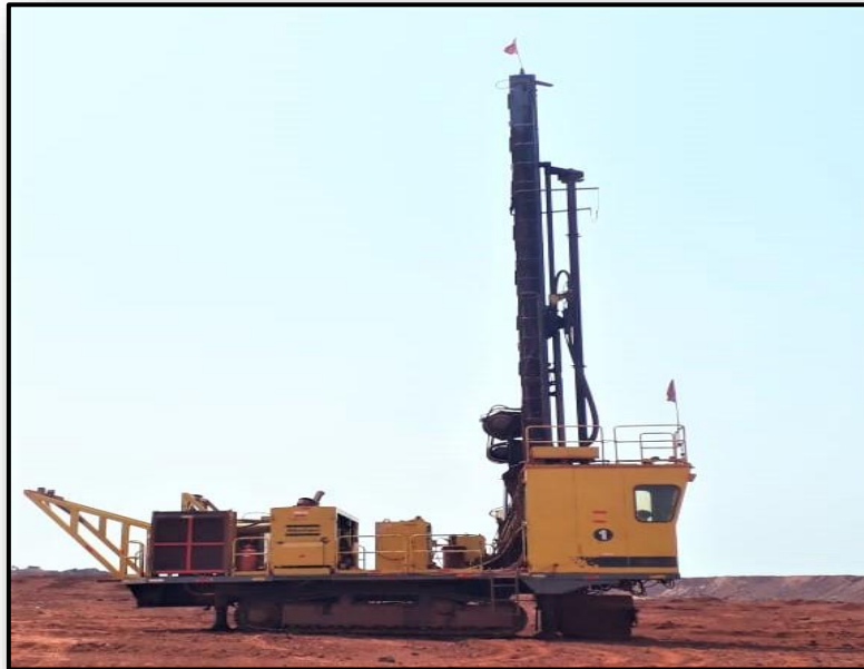
PHOTO 12: Showing drilling machine with dust Extractor.
