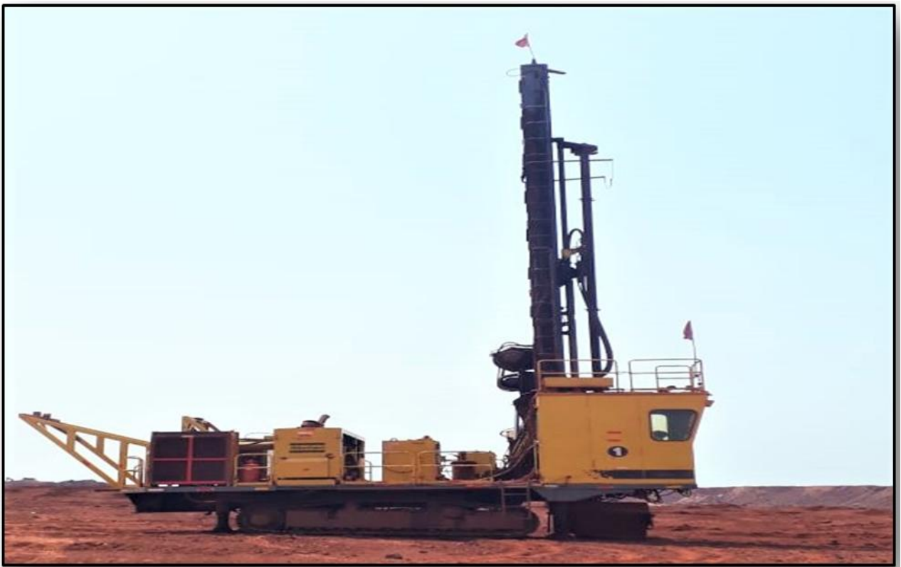
PHOTO 12: Showing drilling machine with dust Extractor.
