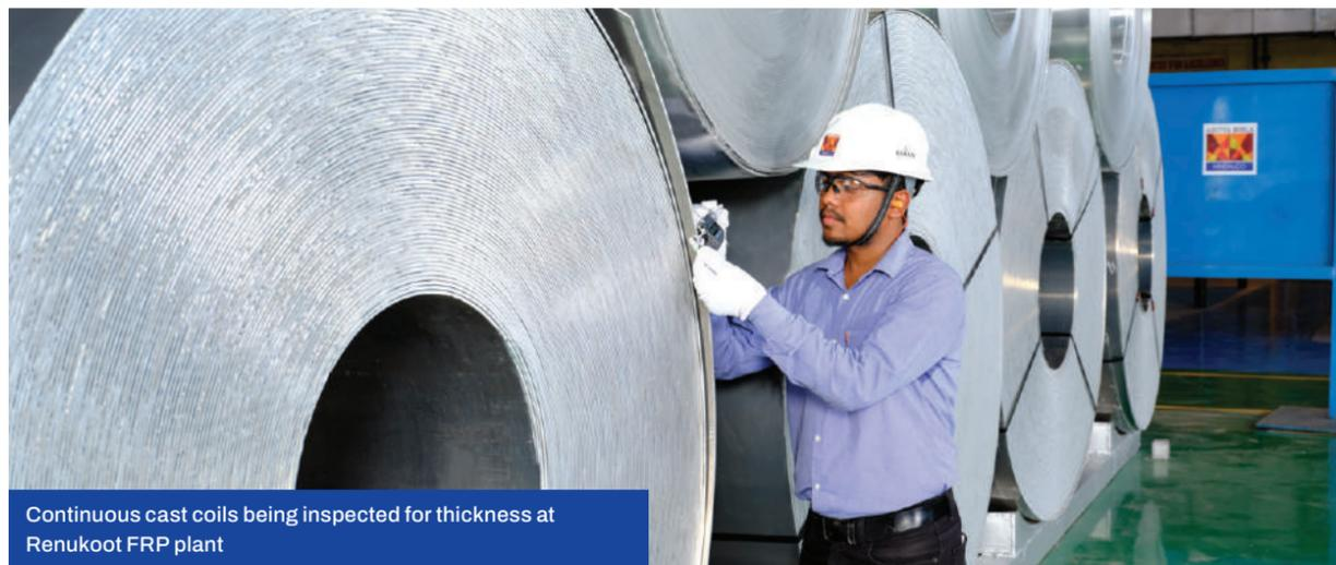
Continuous cast coils being inspected for thickness at Renukoot FRP plant
