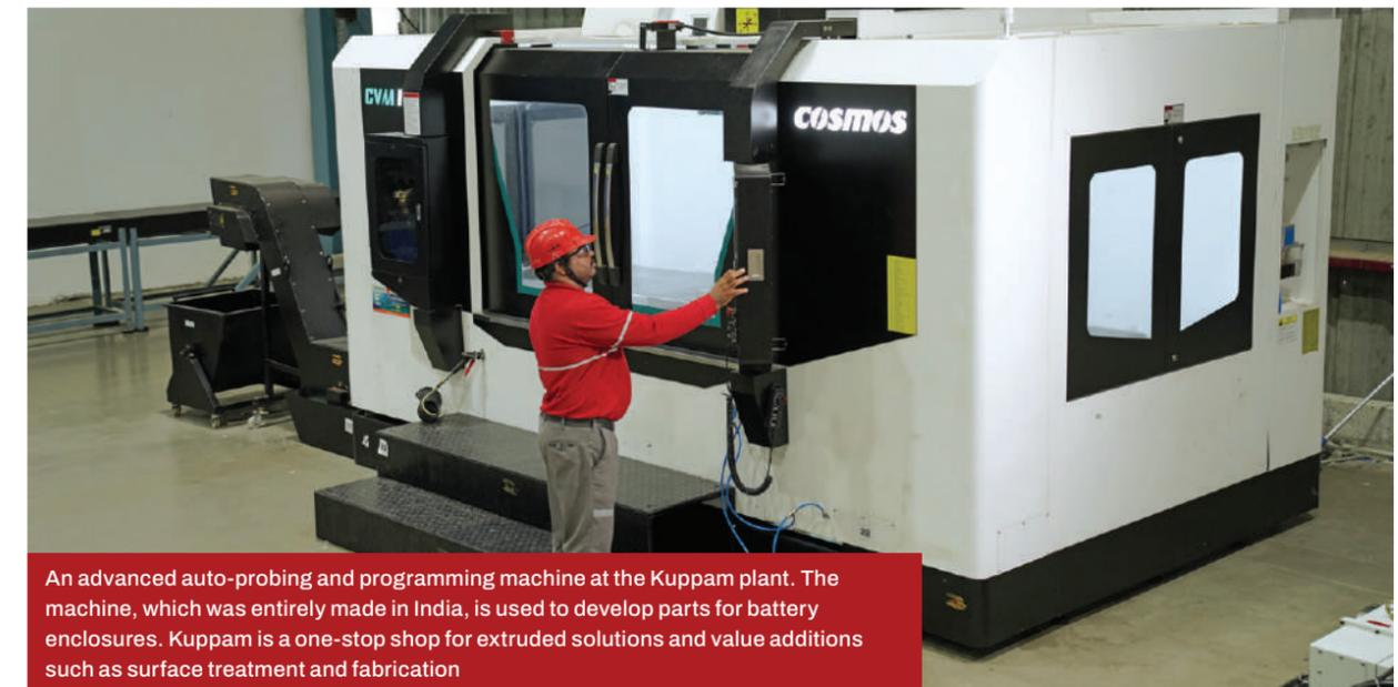
An advanced auto-probing and programming machine at the Kuppam plant. The machine, which was entirely made in India, is used to develop parts for battery enclosures. Kuppam is a one-stop shop for extruded solutions and value additions such as surface treatment and fabrication
