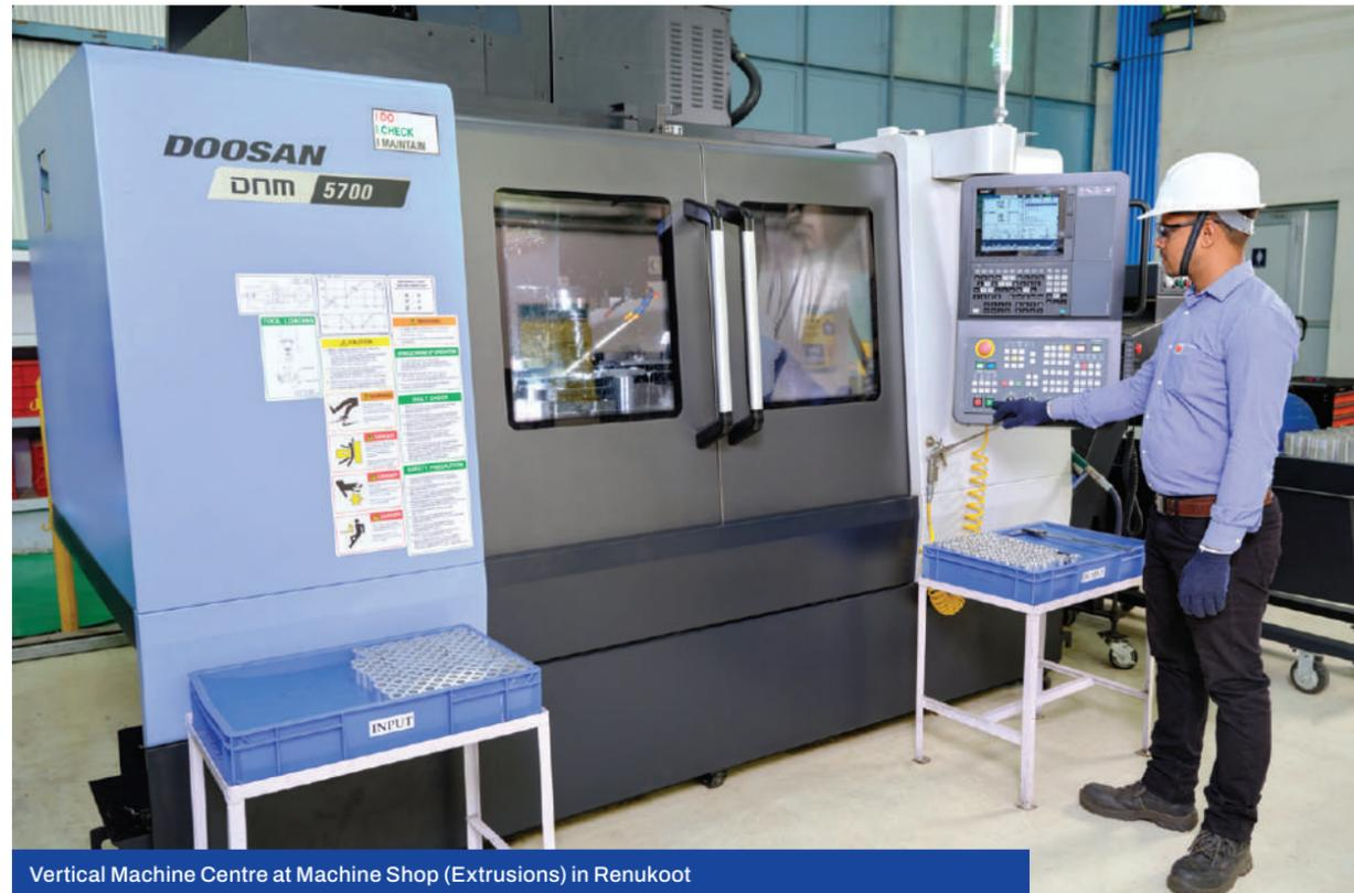
Vertical Machine Centre at Machine Shop (Extrusions) in Renukoot
