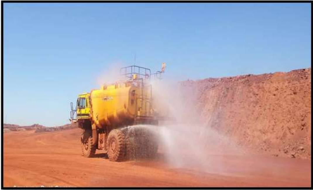
PHOTO 8: Showing 28KL Mobile sprinkler
